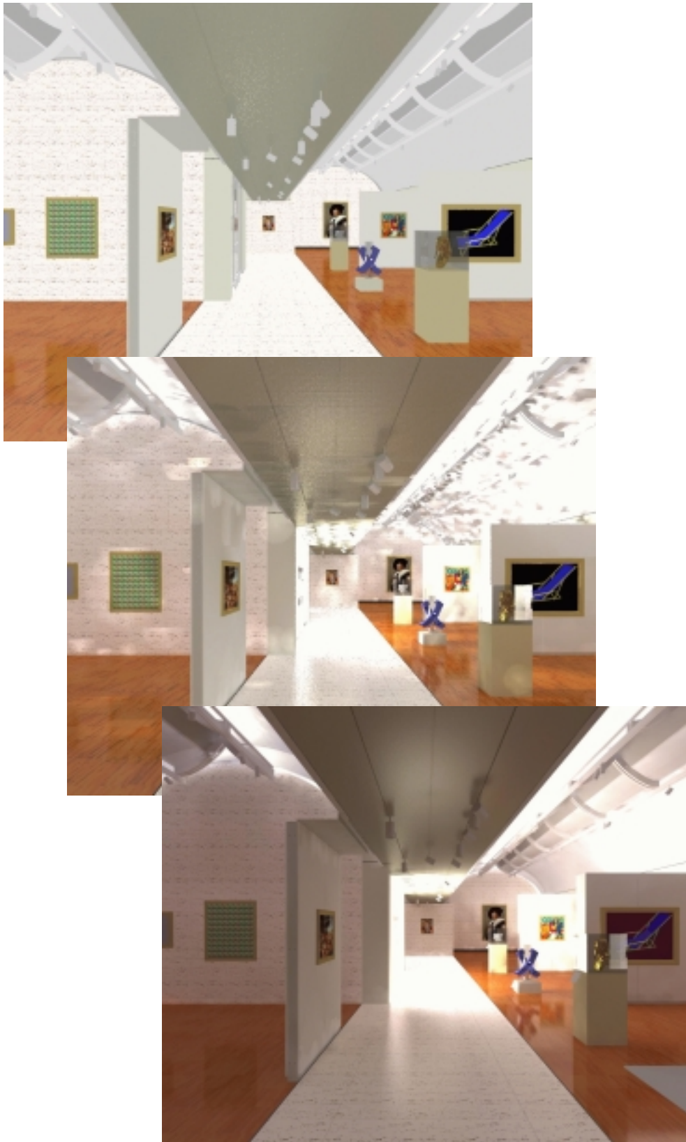
Figure 3.15: Results of three different settings for ambient calculations in Radiance: From top to bottom: constant ambient value (i.e. no ambient calculation, ab = 0 , computation time 0.135 h), one ambient bounce ( ab = 1 , ad = 128 , 0.431 h) and seven ambient bounces ( ab = 7 , ad = 16000 , 24 h). The "mould patches" on the ceilings have disappeared with the higher ad value.
