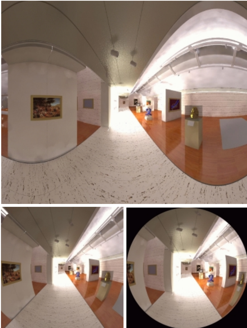
Figure 4.4: Different types of projection of a Radiance image from the same viewpoint: (clockwise from the top: cylindrical, linear fish-eye, cosine fish-eye). A view in parallel projection is not shown here.
