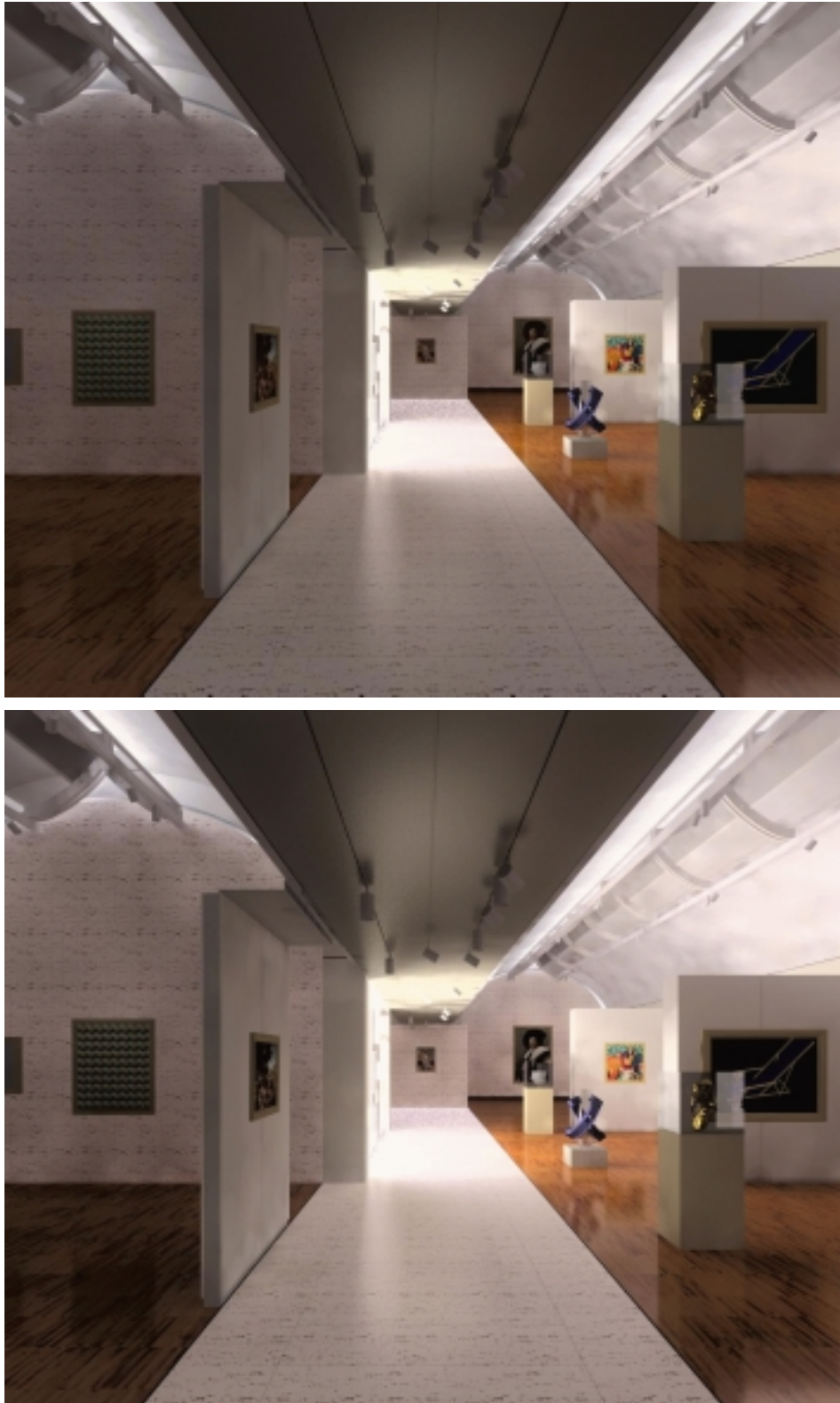
Figure 4.9: The same calculated values as in fig. 4.8, corrected with p_{cond} for reproduction on an output device with maximally 100 \text{ cd/m}^2 and 1:32 contrast. The lower image is also weighted with visual perception parameters (scattering of bright points, scotopic vision).
